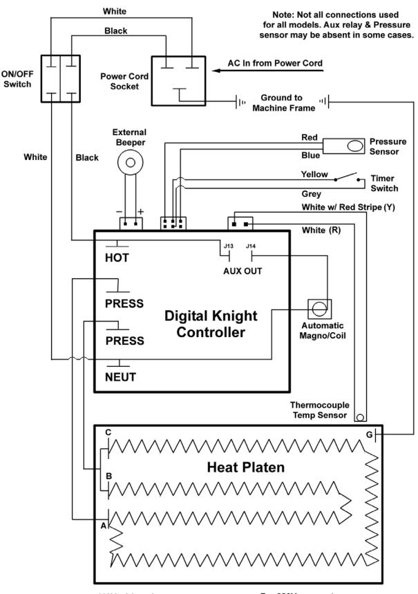
110V wiring shown One power lead to A Other power lead to B & C joined For 220V, connect power leads to B & C, leave A empty
