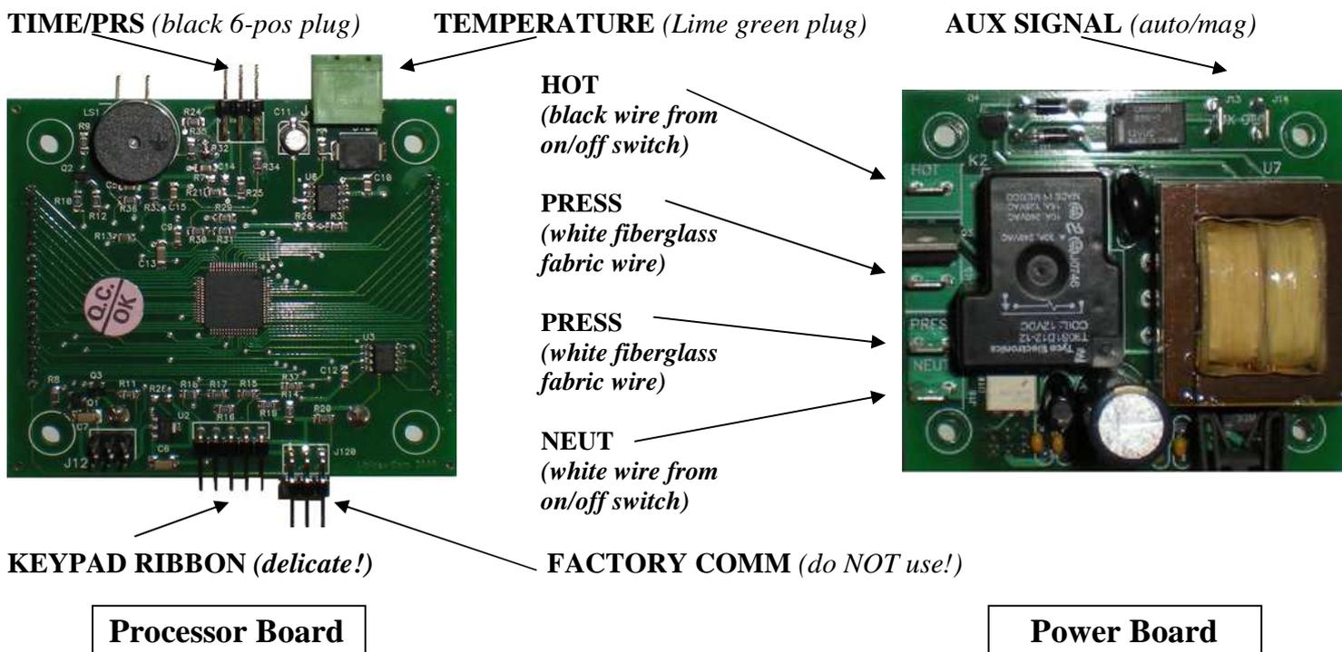
The Digital Knight controller is made up of two circuit boards. One is the Power board, which is visible from the inside. The other is the Processor board, which contains the LCD display panel. When replacing the processor board alone, there is no need to disconnect any wires from the Power board. Follow these steps:
