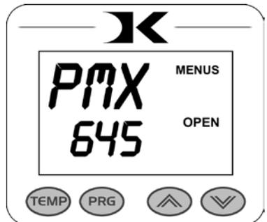
Adjust the pressure of the machine so there is extremely heavy pressure when clamping and locking the press. Press either Arrow Key. The press now considers this pressure as “9” on the Pressure Bar Graph Display.
