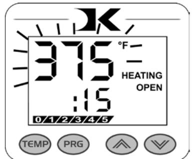
Press TEMP again to lock in the setting. The control will return to the normal operating mode after 10-15 seconds if TEMP is not pressed. 13
