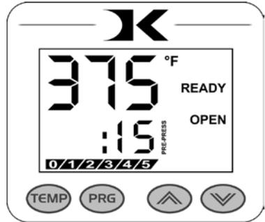
The word **PREPRESS** will be displayed next to the 2nd pre-press time setting when it is active. To set the pre-press time, simply use the Arrow Keys to set the time. If **PREPRESS** is not displayed next to the time, quickly close and then open the press to switch to the prepress time.
