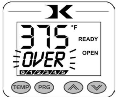
If the OverTemp alarm sounds, turn off the press and let it cool off to room temperature.
