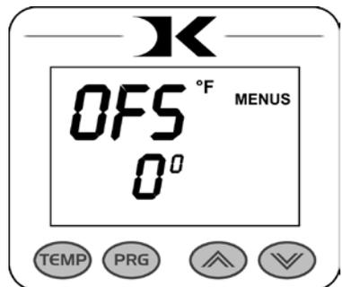
For example: If the controller displays 350°F as the current temperature, and heat platen surface readings are 370, 365, 357, 361, etc, set the offset to +20. The controller will now read 370 instead of 350.
