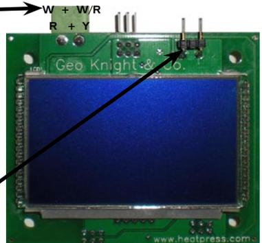
The bottom 6-pin connector is for firmware updates by the factory Only. Do NOT Connect anything to the Bottom 6-pin connector.
