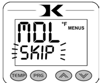
Press PRG and the controller will be programmed with all the settings for the model selected.
