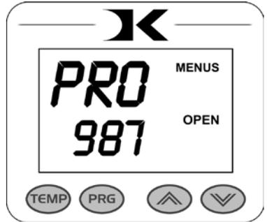
Adjust the pressure of the machine so there is barely any contact or pressure when clamping the press. Press either Arrow Key. The press now considers this pressure as “0” on the Pressure Bar Graph Display.
