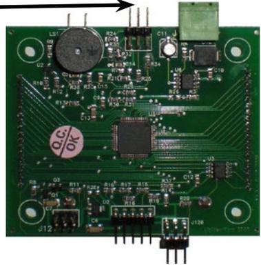
The outer pairs of pins are for the pressure signal. On older models, the height gauge used a red, blue and white wire. On newer models the pressure gauge uses a red and blue wire only. Here is the location for these connections looking down on the pins from the top:
