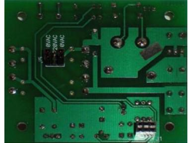
The 6-pin connector mates the 2 circuit boards together. MAKE SURE both boards are oriented to each other correctly to allow this male 6 pin connector to plug into the female 6-pin connector on the LCD board.
