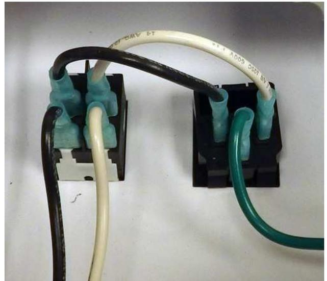
2. Remove small B&W wires. Completely remove the \*SHORT\* black & white wires from the switch and inlet socket and set them aside. ( ← see picture )
