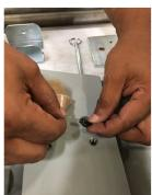
3. Lift up on sensor and pull off the pressure sensor wire harness connector. Plug new sensor into the pressure sensor wire harness so the connector is downward and then pass the connection thru the slot in the base plate. Reverse steps for re-assembly. \*You may need to re-calibrate the pressure settings after replacing the sensor- see the machine's manual.
