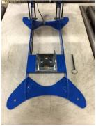
1. Remove the bottom table by pulling out the lower pull pin under the table, and lift the table off. Set the table off to the side.
