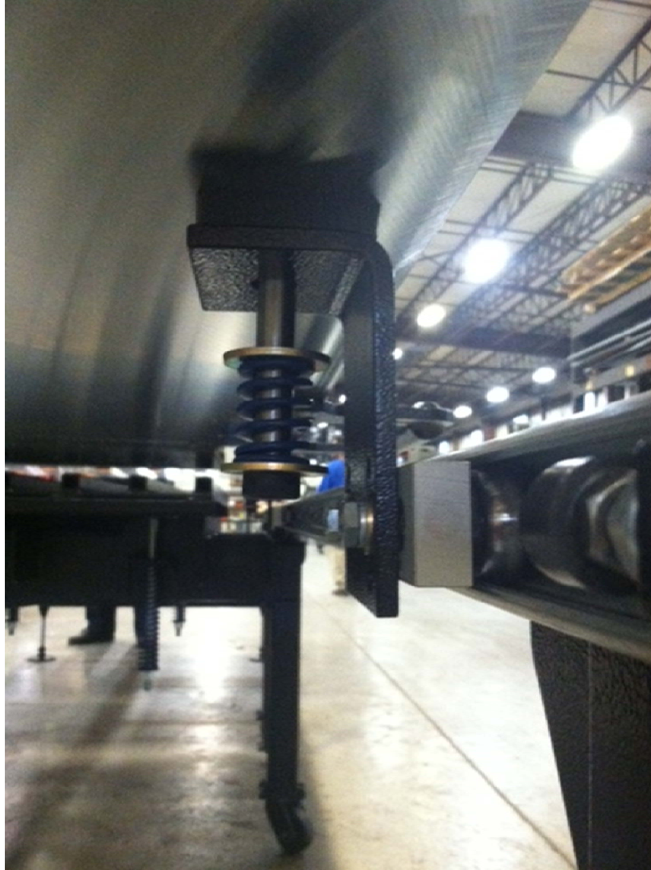
SHOULDER BOLT AND SPRING ATTACHED TO THE ROLLER BEARING ASSEMBLY ENGAGED TO THE RAIL
