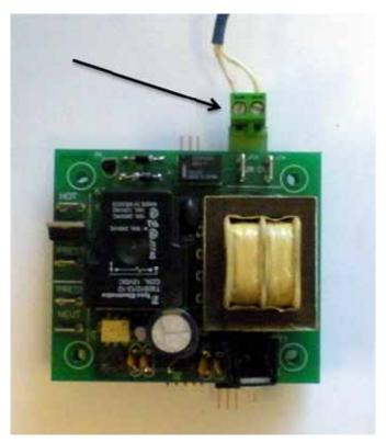
If after unplugging and plugging the lime green connector the Err message still appears; unplug the green connector and remove the 2 tiny wires from the lime green plug. Cut them back 1/4" and strip them so they have new ends. Reconnect them to the lime green plug so they are screwed in tightly and cannot pull out. Plug the green plug back in and turn the press on. Note the picture on the right.
