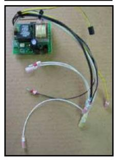
The end of the wire harness with more connections, mixed male & female plugs, connect as follows:
