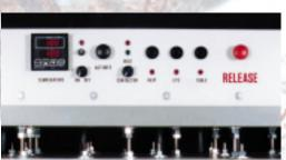
for their longevity, ease of use, and performance. Temperature and timer control units are backed by a 3 year warranty. Indicator lights inform the operator of 'heating' and 'at heat' status. The table switch closed loop activation safety circuit indicates and prevents premature closure.
