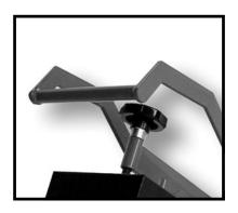
CAUTION: The heat platen will become detached from the frame and drop onto the table if it is adjusted beyond the point of connection.
