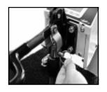
Reconnect the modular connector. An Err display might read on the controller if in the Normal operating mode. If this is the case, once the heat platen is reconnected, turn the machine off and then on again.
