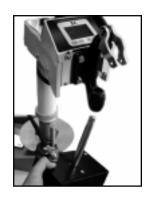
Lift the heat platen into the clamp linkage. Make sure the rear guide fork holds onto the guide pin in the back post of the frame. This holds the heat platen in a straight position and keeps it from rotating.
