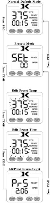
The user options menu is a set of features and calibration options that are programmable and adjustable by the user. It consists of a set of menu items that can be scrolled through. Each menu item is a feature whose values can be viewed and /or changed. To enter the user options menu:
