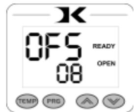
Due to the programming structure of the controller, the offset value will also offset all programmable presets and other stored temperatures. This means that any presets and set point temperatures will need to be set again.
