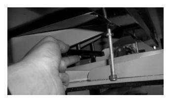
Once the hold-down bar is in place, test the squareness of the shuttle. Swing the heat platen over the shuttle as far as it goes. Slide the shuttle from left to right and make sure the sides of the heat platen are parallel with the silicone pads.
