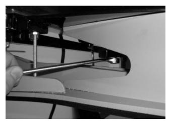
Once this is done, tighten the two nuts against the hold-down bar Very Tightly, to fully secure and lock the shuttle to the base of the press. This is important. Please note the picture shown.
