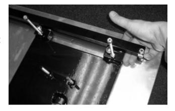
CAUTION: Keep the aluminum shuttle plate centered. Until locked in place, the main aluminum shuttle plate will fall off the press and can cause damage and/or injury if not kept centered. Please note the picture shown.
