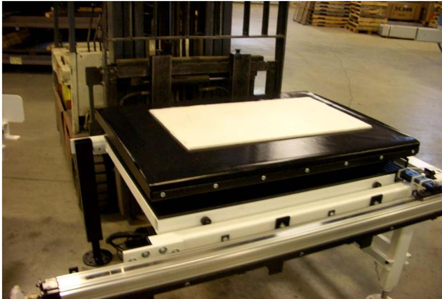
With the extension section lifted off the shipping pallet, now carefully bring the section over to the machine. **MAKE SURE THE NYLON TIES AND THE SHIPPING WOOD IS STILL IN PLACE BEFORE MOVING SECTION.**
