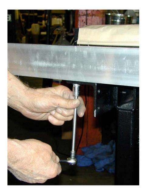
ASSEMBLY OF BASE ROLLER FRAME-Attach the front and rear roller tubes to the (2) angle irons on the maxi base stand. Use the 5/16-18 screws to attached the front and rear roller tubes, then attach the right and left lower side tubes. It would be helpful to use a square on the assembly of this frame to insure proper operation. Try to have the roller frame assembly centered to the lower platen or heater block assembly.
