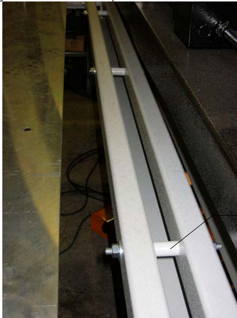
VIEW OF THE (3) SPACER TUBES AND THREADED ROD BETWEEN LOAD VEHICLES
