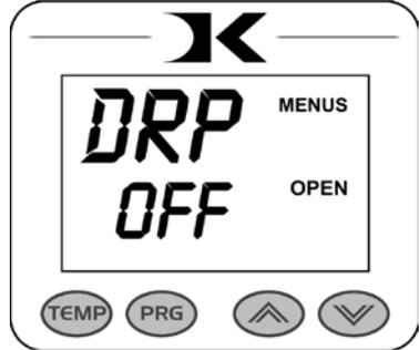
If the current temperature drops below the set temperature by that many degrees, and alarm will sound. Press TEMP to silence the alarm.
