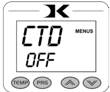
When this feature is ON - the normal countdown timer display is replaced by this odometer instead. The arrow keys no longer adjust the countdown timer, but instead are used to set the countdown odometer. When OFF, the timers are visible.
