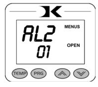
The PPR menu must be set to ON for this menu to be visible. Use the arrow keys to set AL2 to OFF, or 1 through 10.
