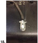
the metal stamp plate and (2) screws on the wire harness metal cord restraint clamp.
