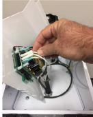
**19.** Reattach heat platen to machine and connect the (2) white fabric heat wires to the male tabs marked (PRESS) on the circuit board. Connect the 3rd white fabric wire that connects to the green ground wire.
