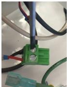
2. Reconnect the thermocouple wires to the green thermocouple connector. (Note wire color orientation SEE PICTURE) Then thermocouple connector to the green thermocouple female on the top edge of the processor board.
