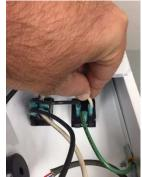
21. Reconnect the BLACK & WHITE wires on the back side of the power socket if you had removed them to determine if you had an issue with the heat platen.
