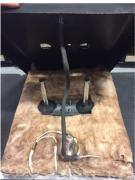
3. Carefully lift the black heat platen cover up while feeding the wire harness thru the harness restraint clamp hole. Once the cover is clear of the wire harness, set it aside.
