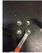
Use the  $\frac{1}{2}$ " wrench or deep socket ratchet wrench to remove the center (4) 5/16-18 nylon hex nuts from the heat platen cover.
