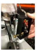
Remove the rear pivot switch box itself from the silver metal stop collar by removing the (2) slotted screws located inside the black plastic box. (Allow the black switch box to hang after removing)
