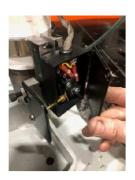
Remove the cover from the rear pivot switch box by removing the corner slotted screws. (Save these screws, you will need these later)
