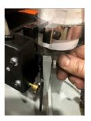
Use the 3/16 Allen Key Wrench to loosen the silver stop collar clamping screw until the stop collar is free to slide up and down on the top white head pipe. Then lift the stop collar/ black switch box up and over the bottom base stop bar and locate the unit in FRONT of the base stop bar. (see picture)
