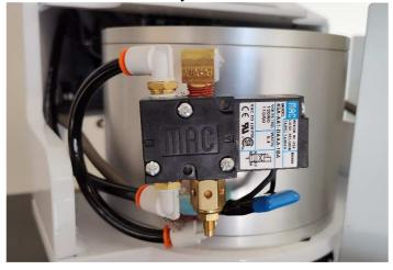
**STEP 3:** On the end of the brass valve, there is a NUT and a Screw. Loosen the locking nut first with pliers or a wrench.
