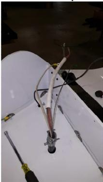
3. Disconnect wires from the heater block that connect to the HEATER RELAY, Green ground wire from ground screw, thermocouple wire from the circuit board. (See Picture)
