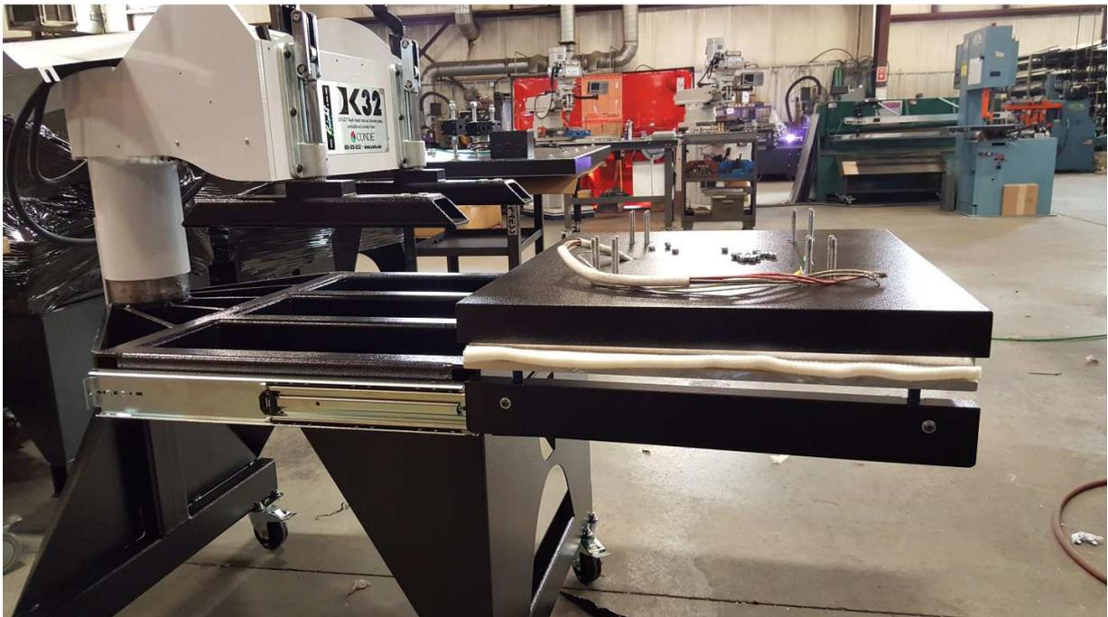
7. Slowly pull out the loading table with the heater block resting on it.
