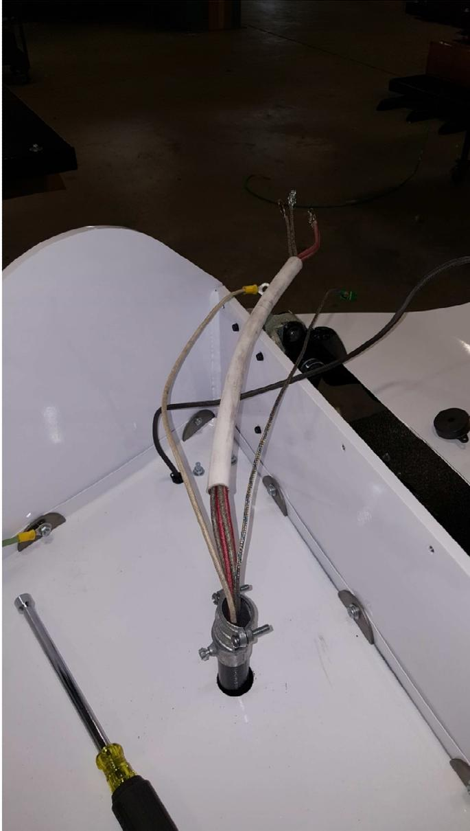
16. With the wires up thru the pipe and cleanly coming out of the upper conduit clamp, re-tighten the (2) clamp screws. Make sure the inner black rubber is in place before tightening.
