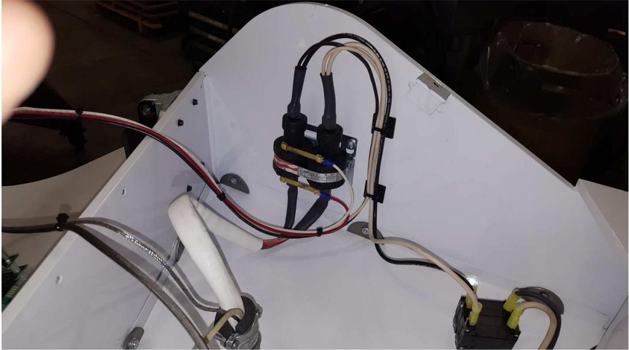
18. Before connecting the heater wires to the HEATER RELAY, pair up the (2) heater wires that are marked with black marker together and slide on the piece of shrink tubing over them. Do the same for the (2) heater wires that are marked with red marker.
