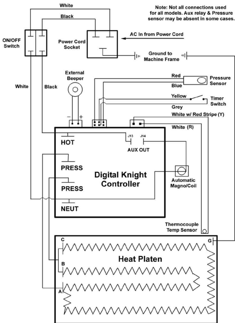
Note: Not all connections used for all models. Aux relay & Pressure sensor may be absent in some cases.
