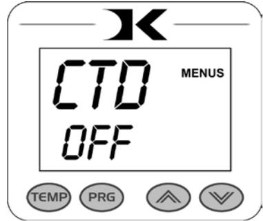
The timer & prepress timer (if ON) still operate. However they are not visible. Instead, at the end of every main timing cycle (but not prepress), the odometer decreases by 1. This way, the operator can keep track of how many pressings are left to do, without checking the REC menu.
