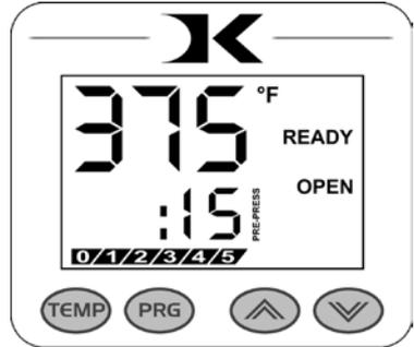
The word PREPRESS will be displayed next to the 2nd pre-press time setting when it is active. To set the pre-press time, simply use the Arrow Keys to set the time. If PREPRESS is not displayed next to the time, quickly close and then open the press to switch to the prepress time.
