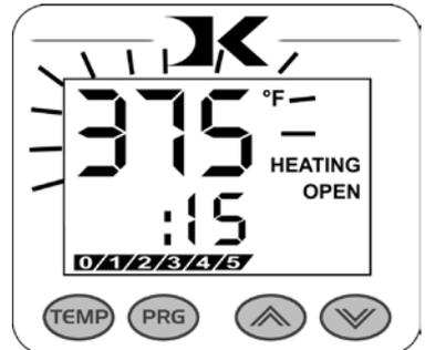
Press TEMP again to lock in the setting. The control will return to the normal operating mode after 10-15 seconds if TEMP is not pressed. 3
