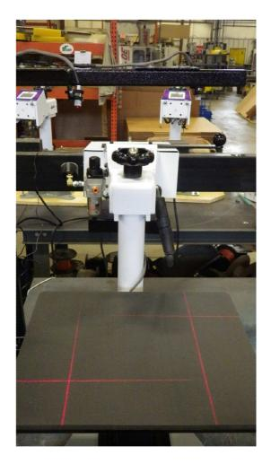
The Laser Alignment System is comprised of a steel mounting frame and laser brackets that allow you to mount laser/s for registration dots or cross hairs on the loading table. The steel mounting frame is designed for you to position next to the machine and bolt or screw into the work bench to secure. The system includes two swivel mounting brackets that give you the ability to locate either a dot or cross hair anywhere on the loading bed.
