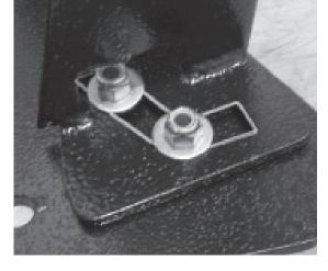
bolt, 4 bolts per caster. One washer under the bolt head, one washer under the locknut. *IMPORTANT: Make sure the nuts are on top, and the heads of the bolts are facing the floor, so the wheels can rotate.*
