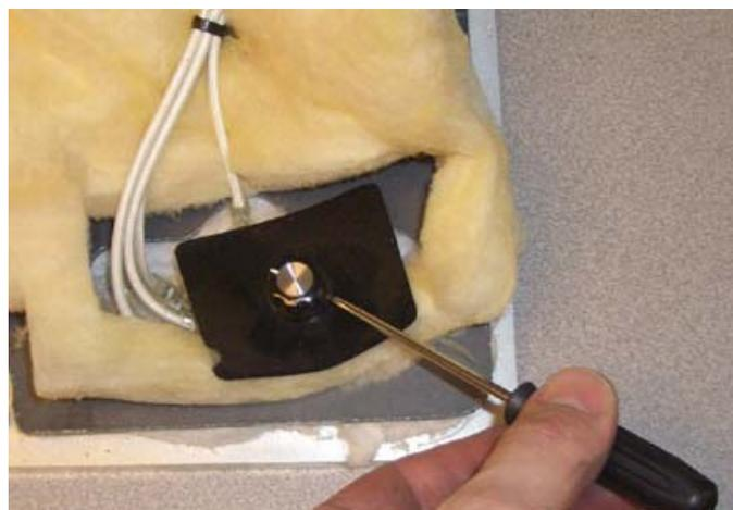
Lay the heat platen cover back over the 4 posts. CAUTION: Make sure the wires are not crimped in the middle of the press, between the cover and the center block. Make sure they are freely travelling from the thermostat and heat element into the top console.
