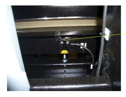
Loading table index lever switch found on rigid table twin left-to-right shuttle machines
