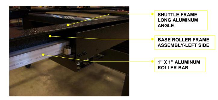
The bolts attaching the Left & Right end tubes lower roller frame may need to be loosened & then tightened while spreading the angles to insure a smooth & tight rolling fit of the Main Teflon Shuttle Frame on the Base Roller Frame Assembly.
