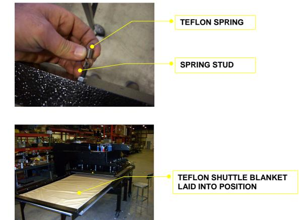
With the Teflon blanket now secured, shuttle the assembly to the left and right. Make sure that the Teflon slides smoothly without risk of abrasion against edges or surfaces. In most cases the bottom heater block will have a layer of 1/8" green heat conductive rubber laying on top of the heater block surface. The Teflon blanket needs to be above this green heat conductive rubber/semi porous Teflon by approximately ½".
