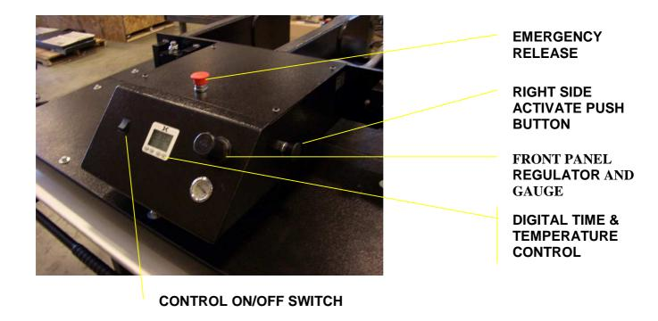
**LCD TIME AND TEMPERATURE CONTROL:** Please refer to the KNIGHT DIGITAL CONTROLLER MANUAL for proper operation of the digital controller.
