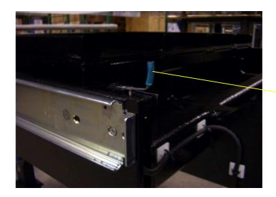
Loading table index lever switch found on all single station front loading machines
